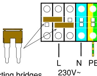
The terminal connection block is accessed after removing the boiler front panel . The supply cable should be safely routed to this point through the cable entry point on the right hand bottom of the boiler.
