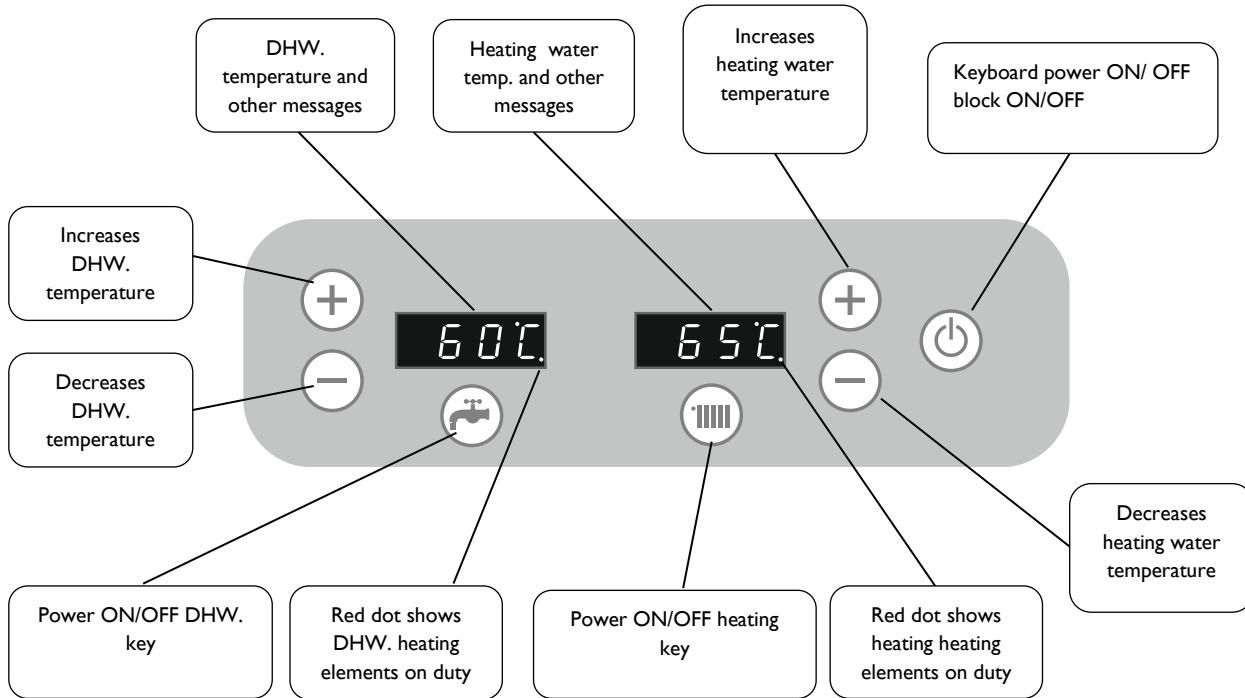
Push the button to start the boiler up. The same button will turn the boiler off when pushed again.
